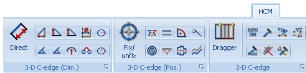
Fig. 91 Edge constraints (if sketch is active)
