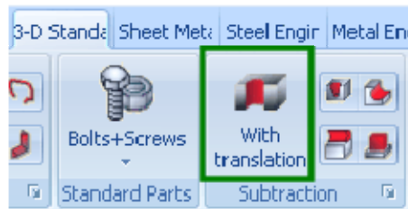
Fig. 102 3-D Standard tab, Subtraction function group
