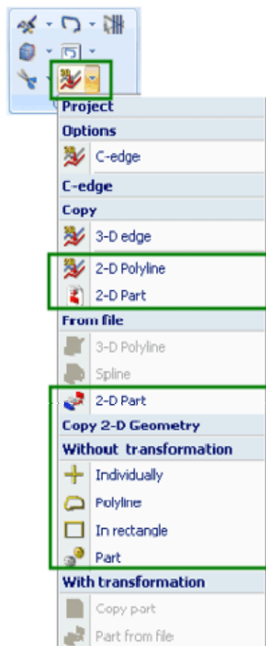
Fig. 88 Functions for the copying of 2-D lines into sketches (to convert 2-D to 3-D)
