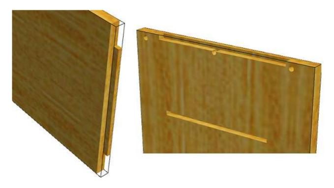
This version allows you to assemble two parts while avoiding horizontal drillings in the edges.
